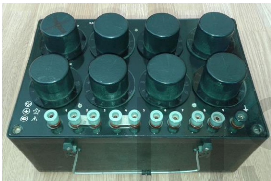
Fig. 1. General view of P4834 resistance decade box
